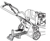
• Replace the blade with the supplied Combi blade. For more information, see "Cutting equipment".
