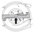
Lock the blade with a wooden block. Fit the washer and tighten the bolt correctly by turning clockwise. The bolt should be tightened with a torque of 70 Nm.
