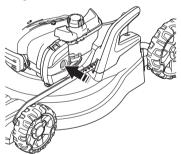
The engine brake handle must be held against the handlebar when the engine is started.
