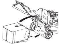
Fit the bagger bottom in the discharge hole.
